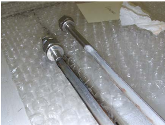
Figure 5 Comparison of untreated (right) to PWT treated tube (left)
