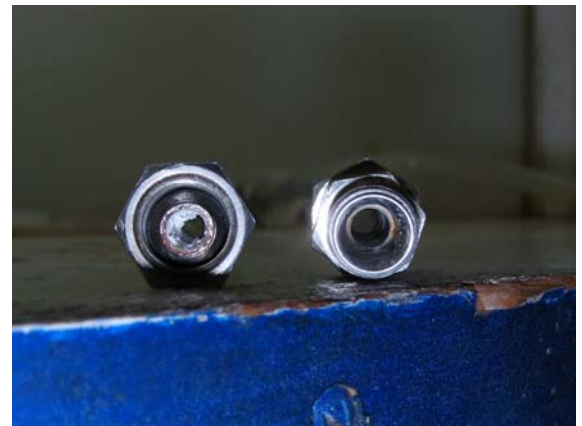
Figure 6 Untreated tube (left) and PWT treated tube (right)
