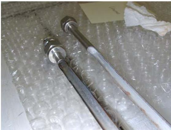
Figure 5 Comparison of untreated (right) to PWT treated tube (left)
