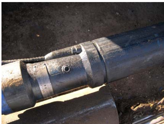
Figure 11 ESP has no scale
