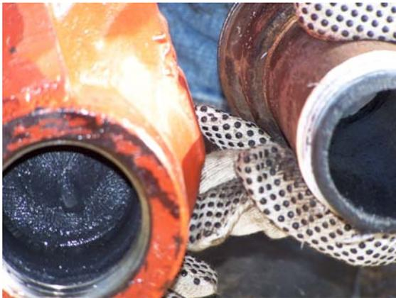
Figure 13 Inlet and discharge of check valve clear of scale after 8 months
